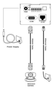
Shut down all the peripheral devices prior to connection. Connect the supplied cables from VisualServer to related devices according to the following steps. Note that the power adaptor must be kept unplugged until other cables are firmly connected.
